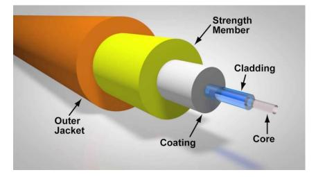
Light path spreads along fiber because of <u>total internal</u> <u>reflection</u> which happens due to different indices of refraction
